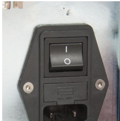
Figure 6: CM rocker switch in the “I” position representing power as ‘ON’
