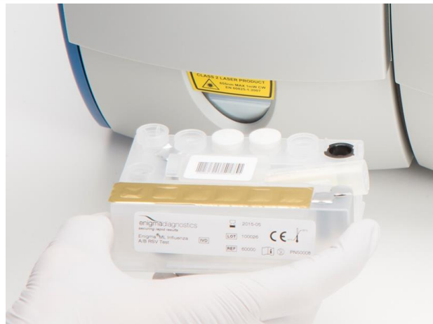
Figure 18: Capturing cartridge ID by scanning barcode from the centre of the test cartridge
