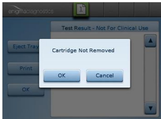
Figure 38: Alert screen prompting the operator to remove the spent test cartridge before returning to the main screen
