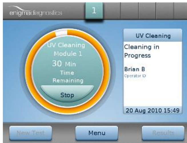
Figure 32: UV cleaning protocol display
