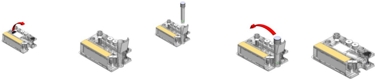
Figure 16: Illustrations demonstrating an overview of sample & cartridge loading
