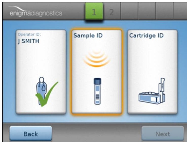
Figure 14: Screen showing a successful Operator ID has been captured & prompt for the Sample ID
