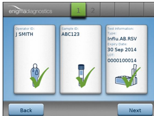
Figure 19: Screen indicating all three IDs have been successfully entered
