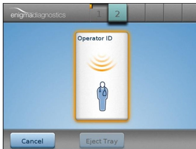
Figure 31: Scan operator ID display to start UV cleaning protocol
