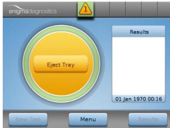
Figure 37: Reporting that an error in PM 1 has occurred, prompting the operator to eject the tray
