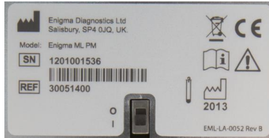
Figure 5: PM platform label & PM isolator switch in the “I” position representing power as ‘ON’
