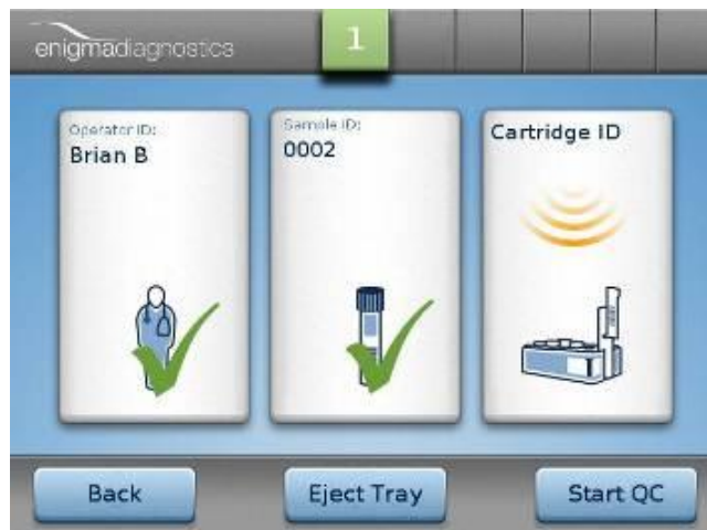
Figure 17: Screen showing successful Operator ID & Sample ID entry & prompt for the Cartridge ID
