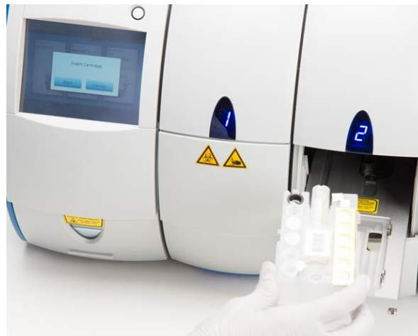
Figure 21: Correct loading of the cartridge into the extended tray
