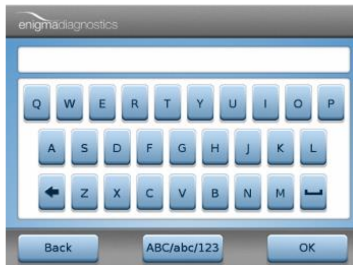
Figure 13a: The QWERTY keyboard for the manual data input ( N.B: delete key bottom left, space key bottom right)
