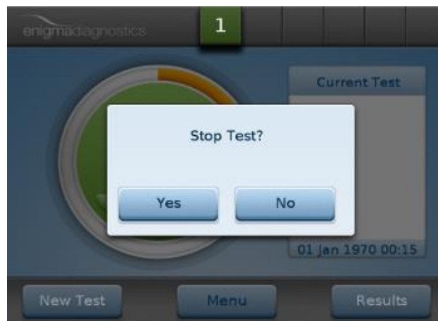
Figure 25: Confirmation screen to confirm test stop
